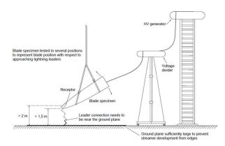
Figure 5. High Voltage (HV) initial leader attachment test.
