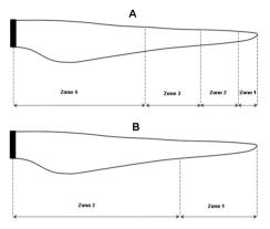
Figure 3. Examples of generic blade lightning environment definition
