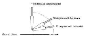
Figure 6. Blade Orientations for initial leader attachment tests.
