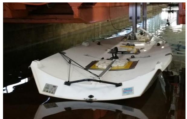
Figure 4 Full-scale Musto Skiff in Tank
