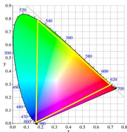
Fig. 5. The gamut of the RGB laser system [17]
