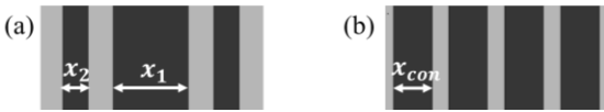
Fig. 2: Schematic diagram of a single element within the array. (a) Level II CS fractal; (b) 2-2 piezocomposite (Black: Ceramic; Gray: Polymer)
