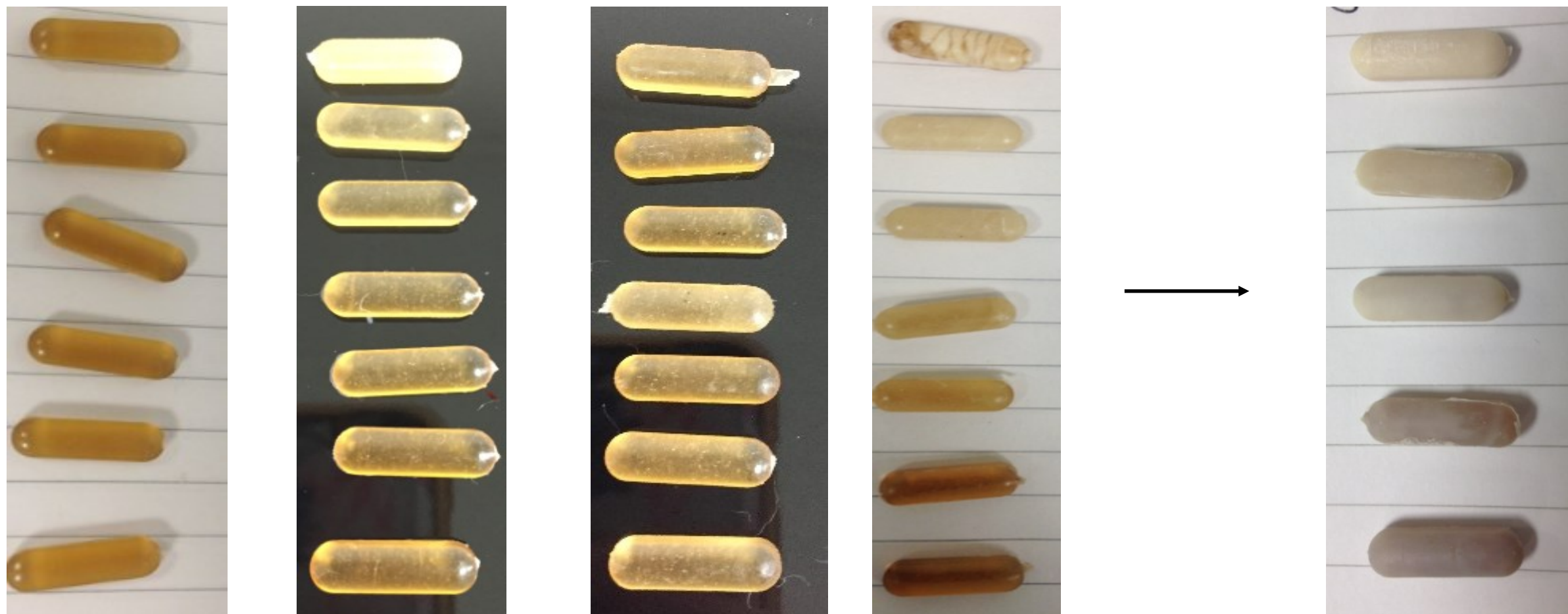
Figure 1: Dosage forms produced using HME-IM using the polymer affinisol and paracetamol (PCM) concentrations 5, 10, 20 and 50% (left to right), followed by 50% PCM formulation which recrystallised during storage
