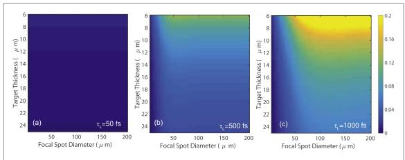
**Figure 5.** l– $\phi_L$  parameter space plots. The colour maps corresponds to the difference in total energy between the input and output spectra for  $\tau_L$  equal to: (a) 50 fs; (b) 500 fs; (c) 1000 fs.
