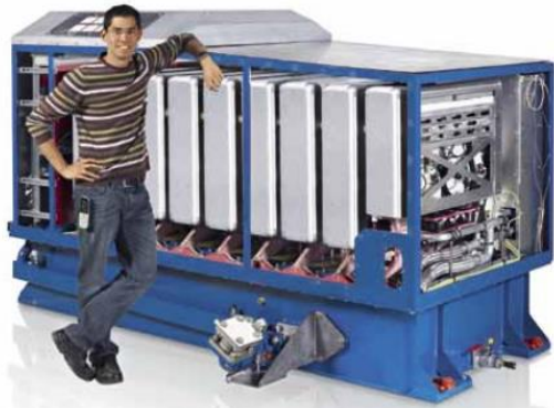
Figure 4: Transformer and rectifier device shown to indicate scale 51
