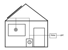
Figure 6: The situation for net-metering.
