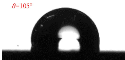
Fig. 9. Water droplet on the smoothly milled surface.
