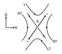
Fig. 2: Schematic hyperbolic fixed point E with stable (-) and unstable manifolds (+), transit (T) and no-transit (NT) phase paths.
