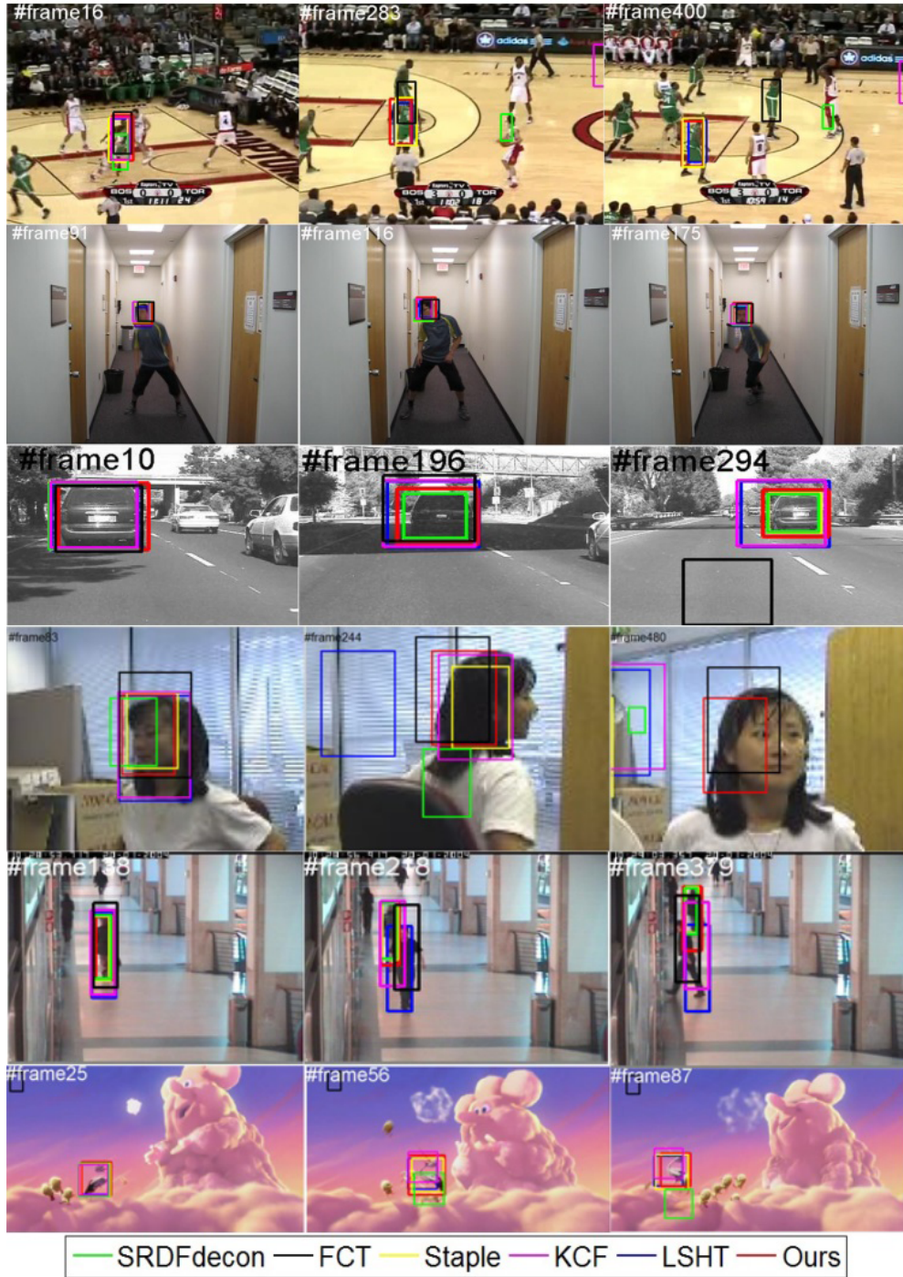
Fig 8 Tracking results comparison of the tested videos on some key frames, where the tracking results are represented as a bounding box. Different color represents different tracker.
