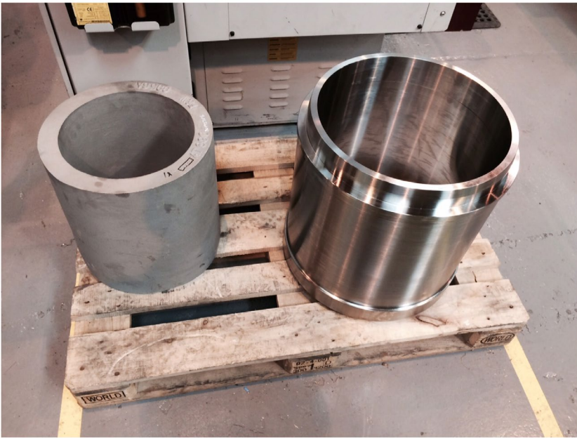
Figure 6. Centrifugal casting blank (left), semi-finished valve cage (right).
