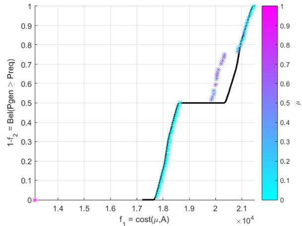
Figure 3: Reliability Pareto front obtained for the design problem in its bi-objective formulation superposed to the exact Belief curve of the worst-case optimum (black line). Colours relate to the proportion of cells of type I and II.
