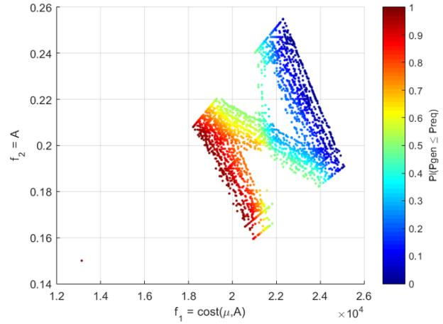
Figure 5: Reliability-budget Pareto Front obtained for the design problem in its three-objective formulation projected to the budget axis, colours relate to the reliability index.
