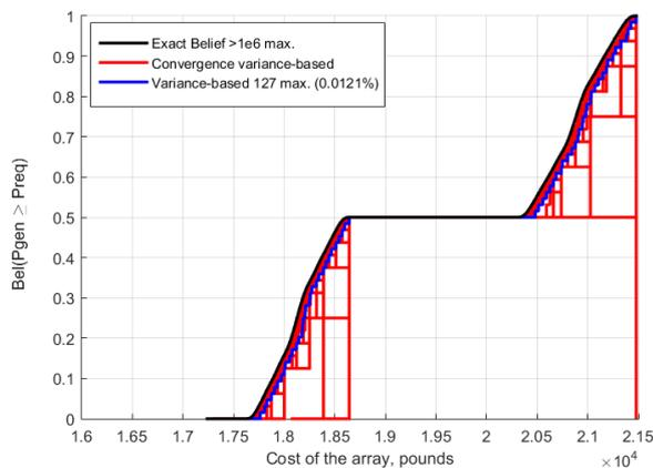
Figure 2: Progressive approximation of the exact reliability-budget curve of a design solution composed entirely of cells of type II ( $\mu = 0$ ). Highlighted, the approximation corresponding to 7 iterations yielding 127 maximisations, i.e. 0.0121% of the computational cost of obtaining the exact curve.
