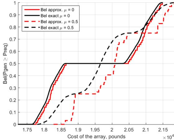
Figure 4: Reliability-budget curves of design solutions with  $\mu = 0$  and  $\mu = 0.5$ . Both the exact curves and those obtained with 7 iterations of the variance-based estimation algorithm are shown.
