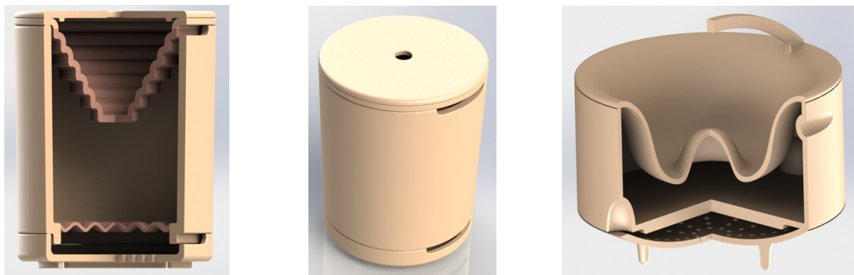
Figures 15-17 Renders of final ceramic filter design for initial tests in Malawi
