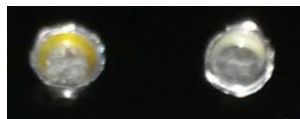
Figure 43: DSC pans containing hydrocortisone (left) and PEG4000 (right) after exposure to over 210°C and 60°C respectively
