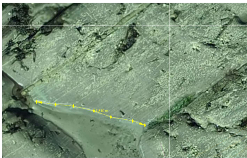
Fig. 5 The length of a joint could be specified with at a level of detail better than 1 cm. (Tziavou, 2016)
