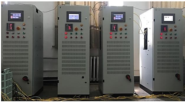
Fig.13. Experimental platform of four-terminal VSC-HVDC test grid.
