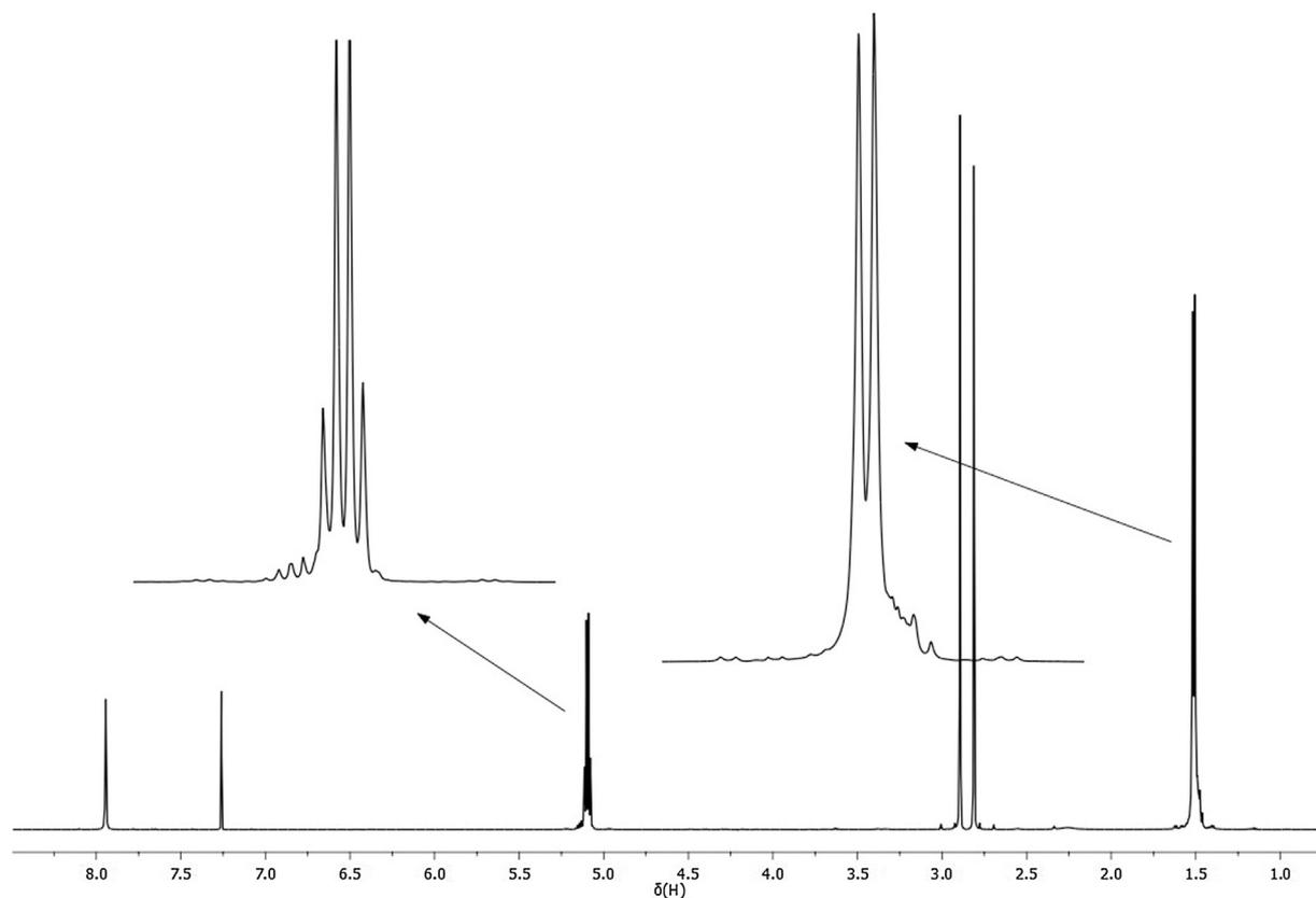
Fig. 1. The <sup>1</sup>H NMR spectrum of poly(lactic acid) in CDCl<sub>3</sub>:DMF, 95:5, V/V%.
