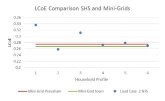
Figure 9. Comparison of SHS solution and using mini-grid for lighting only case.
