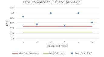
Figure 11. Comparison of SHS solution and using mini-grid for all electrical appliances case.
