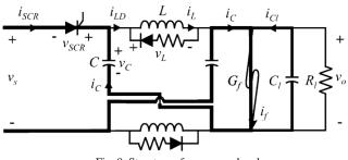
Fig. 8. Structure of a z-source breaker
