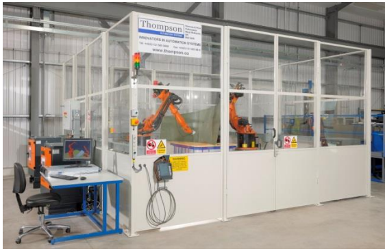
Figure 1: The IntACom Robot Inspection cell showing a large component under test
