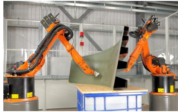
Figure 1: The IntACom Robot Inspection cell showing a large component under test
