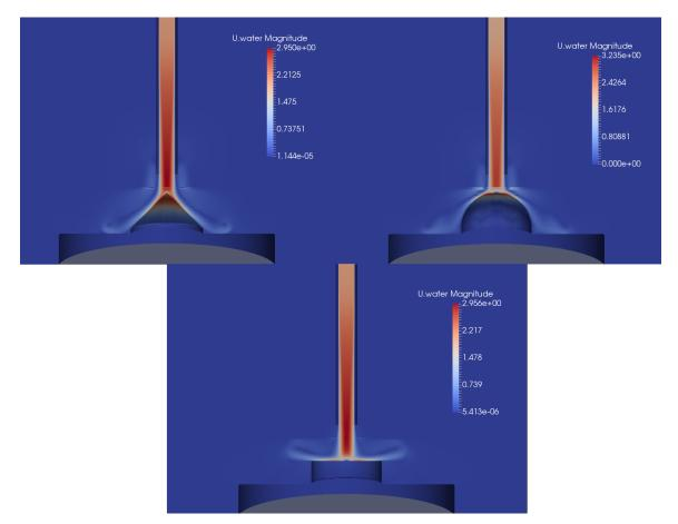
Figure 2: First phase velocity contours. Clockwise from top: cone, hemisphere and cylinder
