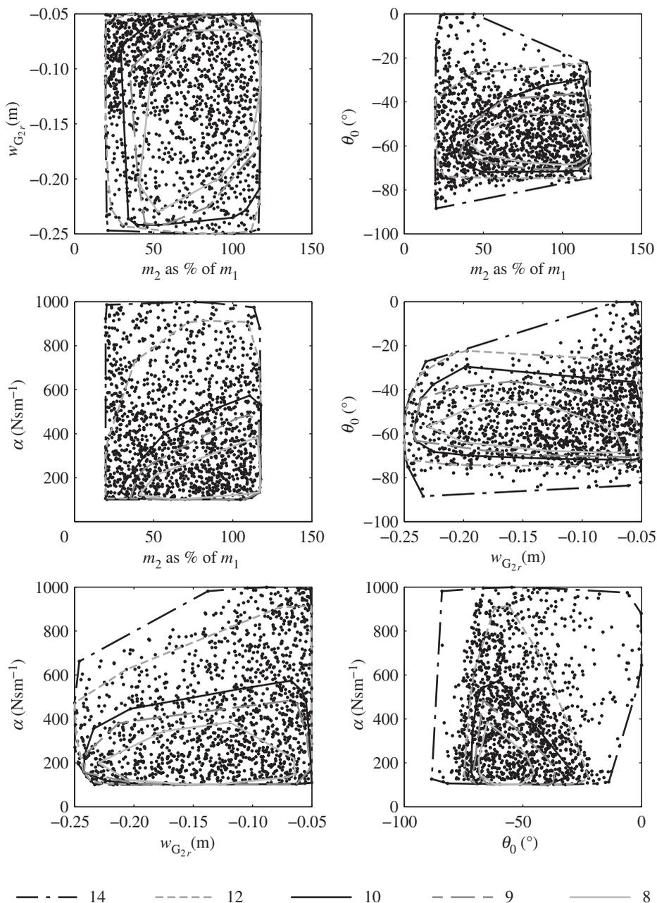
**Figure 1.** Experimental plan. Each dot represents one of the configurations from the dataset trimmed with a motion threshold of 14. The different lines correspond to the extent of the dataset trimmed by motion thresholds of 8, 9, 10, 12 and 14.
