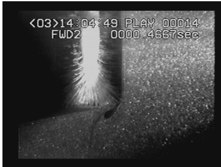
Figure 2 Seeded flow laser illuminated image
