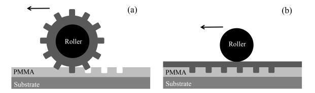
**Fig.3** Schematic picture showing the roller NIL methods as perceived: (a) cylindrical mold method and (b) flat mold method [28]
