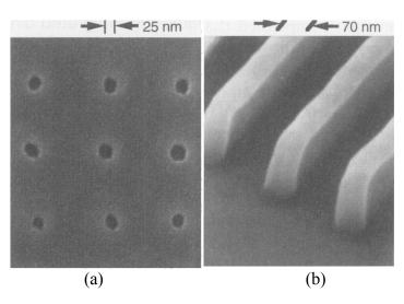
**Fig.2** Scanning electron microscopy image of a (a) PMMA film having 25 nm hole structure (top view), (b) strip pattern formed on a PMMA film using the imprinting process (perspective view) [10] (Reprinted from ref. [10] with permission)
