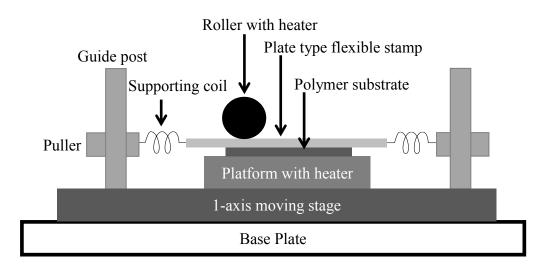
Fig.5 Schematic picture showing the thermal roller NIL approach [32]
