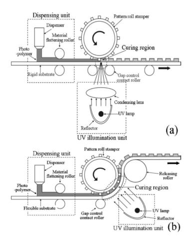
**Fig.**7 Schematic diagrams of the UV roll nanoimprinting system: (a) for a rigid substrate and (b) for a flexible substrate developed by Ahn et al. [33] (Reprinted from ref. [33] with
