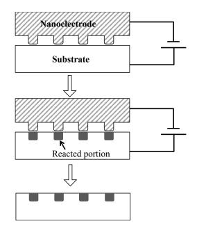
Fig.10 Principle of NEL [51]
