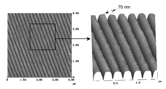
**Fig.4** PMMA nanostructure of sub-100 nm resolution created using roller imprint method [28] (Reprinted from ref. [28] with permission)
