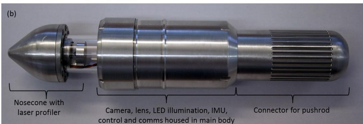
Figure 2 (a) Example of laser profiler image. (b) Laser profiler and camera geometry.
