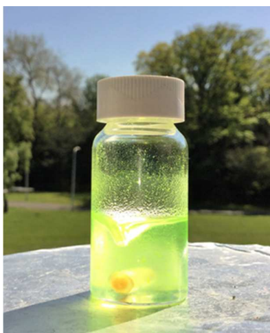
33 34 Figure 6. Experimental set-up of the conversion of \alpha -terpinene to ascaridole using ^1\text{O}_2 produced 35 from direct sunlight irradiation. 36 37
