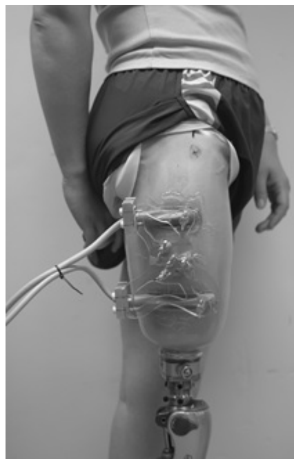
Figure 4: Transducer array in situ .
