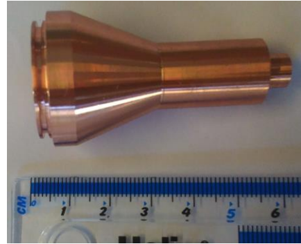
Fig.3. machined profile horn without been brazed with vacuum flanges.
