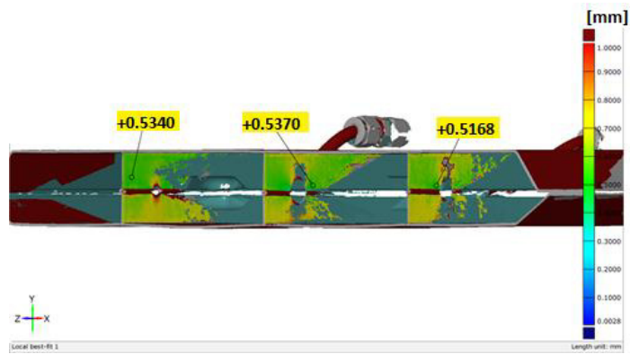
Figure 6 GOM scanning to identify the thinnest spot at inter-cell wall of pack #5
