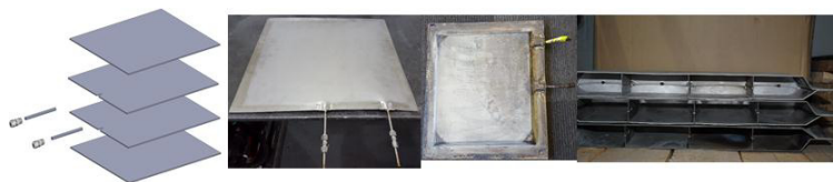
Figure 3 Different stages of the multisheet packs during the manufacture and investigation processes.
