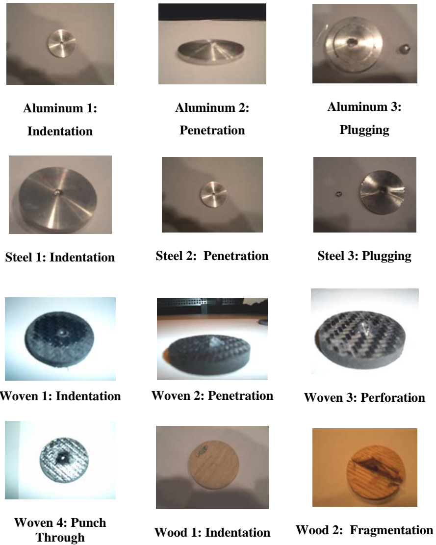
Fig. 3 Images of different damage modes in the tested samples of aluminum, steel, woven composites, and wood
