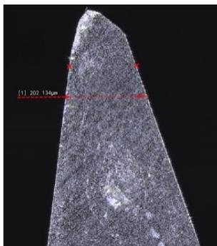
Fig. 4. Flat V-shaped tool (after micro milling)
