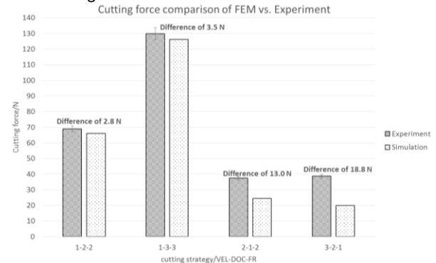
Figure 3. Cutting force comparison between FEM and experiment. It can be seen, that the simulation results agree well with experiment. However, the simulation result is lower than the experimental results. The bigger difference in experiment 2-1-2 and 3-2-1 is possible caused by the inconsistency of work materials used in the experiment as well as wear on the cutter which is neglected in the FE model.
