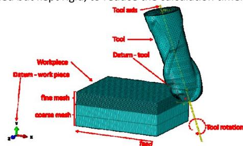
Figure 1. FEM milling model setup
