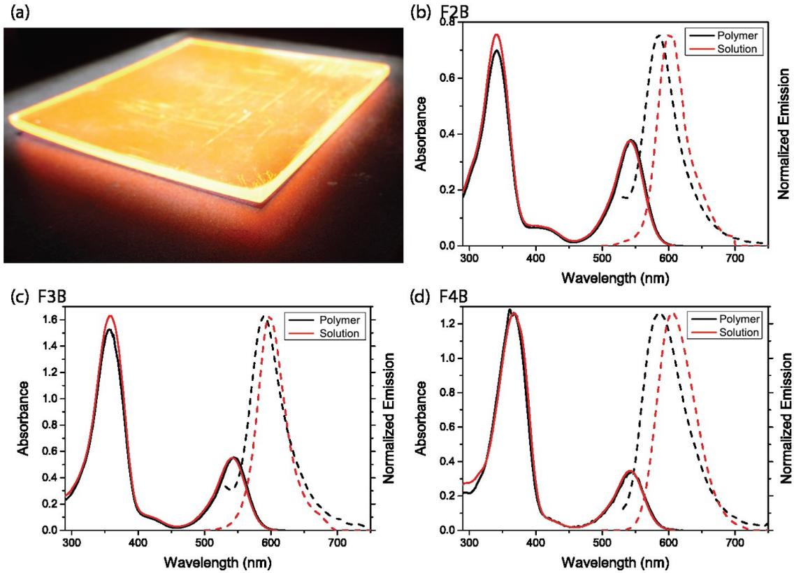
Figure 3: (a) LSC (F2B) photoexcited at 365 nm. Measured absorption and normalized emission of the LSCs (b) F2B, (c) F3B and (d) F4B.
