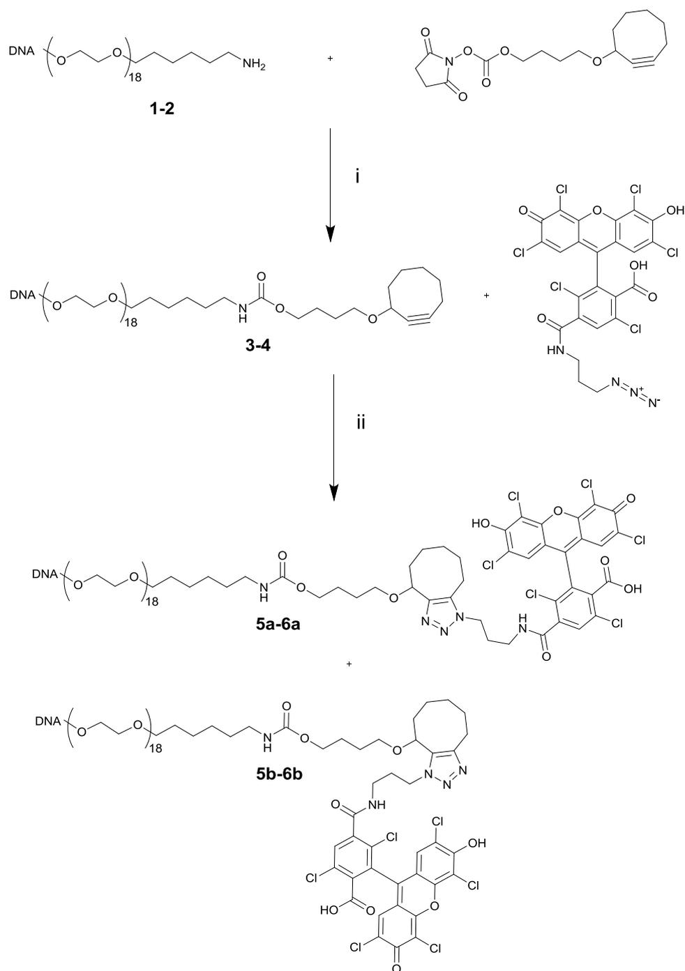
**Scheme 1.** Synthesis of DNA cyclooctynes 3-4 and their conjugation with 4-((3-azidopropyl)carbamoyl)-3,6-dichloro-2-(2,4,5,7-tetrachloro-6-hydroxy-3-oxo-3H-xanthen-9-yl)benzoic acid. Reagents & conditions: (i) 0.025M NaHCO<sub>3</sub> buffer, CH<sub>3</sub>CN, RT, 12 hrs. (ii) 4-((3-azidopropyl)carbamoyl)-3,6-dichloro-2-(2,4,5,7-tetrachloro-6-hydroxy-3-oxo-3H-xanthen-9-yl)benzoic acid, CH<sub>3</sub>CN-DMSO, 24 hrs.
