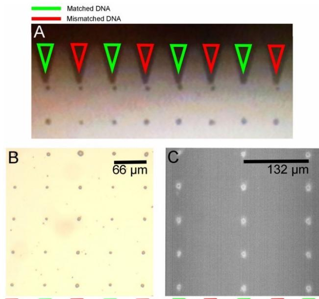
**Fig. 4.** Sequence-selective binding of zfRC-LH1 to matched and mismatched dsDNA using dual-sequence DPN. (a) DNA printing using pens to create alternate 5 μm spots of matched (green) and mismatched (red) DNA. (b) Bright field image of the printed DNA array. (c) Fluorescence image of the pattern after ZF-RC-LH1 binding to DNA. Each row is spaced 66 μm apart. Excitation: 532 nm. Emission: > 650 nm.
