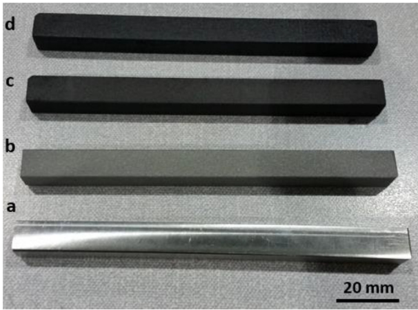
Fig. 4. Billet appearance after different steps of billet preparation (a) 1st step – initial machined billet, (b) 2nd step – sand blasted billet, (c) 3rd step – graphite coated billet and (d) 4th step – anti-seize lubricant applied.
