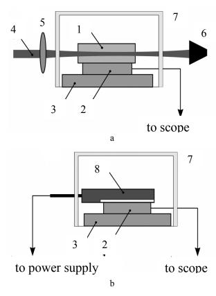
*Figure 1* – Schematic diagram of the set-up used for the calorimetric measurements of loss (a), and for calibration of the set-up (b)
