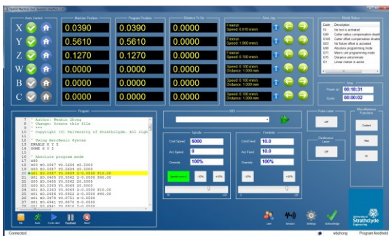
Fig. 5 An example of customised human-machine interface
