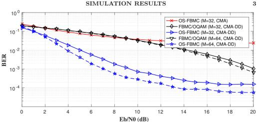
FIGURE 2. BER performances comparison of FBMC/OQAM to OS-FBMC
