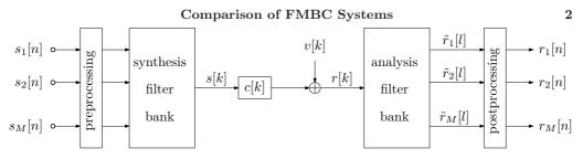
FIGURE 1. Block diagram of a general FBMC system.
