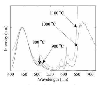
Figure 6. Normalised emission spectra of screen printed BAM:Eu single-layer coatings after heat treatment in air at 800 °C, 900 °C, 1000 °C and 1100 °C.
