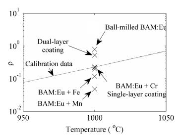
Figure 11. Intensity ratio of various mixtures of commercial powder and transition metal ions, the ball-milled powder and single and dual-layer coatings.
