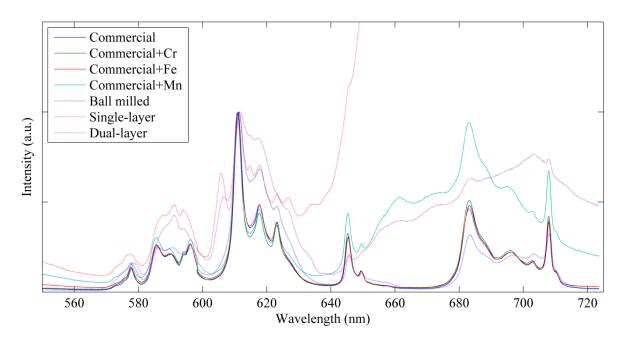
Figure 8. Normalised emission spectra of Eu<sup>3+</sup> of various mixtures of commercial powder and transition metal ions, the ball-milled powder and single and dual-layer coatings.
