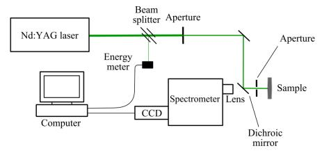
Figure 1. Schematic of luminescence detection set-up.
