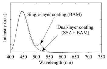
Figure 10. Normalised emission spectra of as-synthesised single and dual-layer BAM:Eu coatings.
