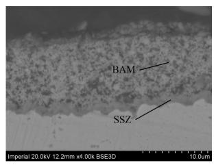
Figure 9. SEM cross-section image of the BAM:Eu screen printed coating with an interlayer of SSZ.
