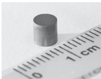
Figure 4. A formed sample (solid cylinder) with a size of \Phi 4.0 \text{ mm} \times 4.0 \text{ mm} .
