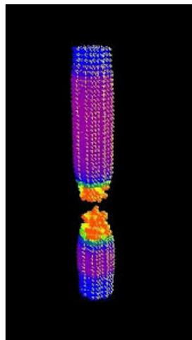
**Fig. 4.** A meshless discretization for a peridynamic model of a cylindrical bar under tension loading [18]
