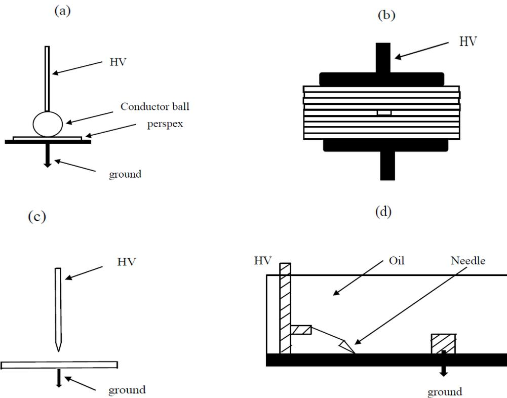
527 Fig. 1: Simulated PD faults a) surface discharge in air b) single void in PET c) corona in air d) surface
