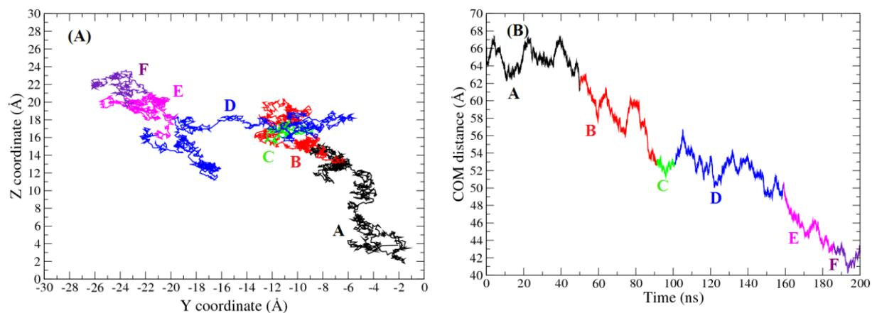
**Figure 3.** The CoM movement of the protein during the adsorption simulation: (a) plan view of the surface; (b) side view showing separation from the surface plane. The different stages of the adsorption trajectory are labeled.
