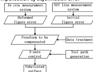
Figure 2 Schematic of compensation procedure
