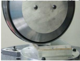
Figure 3 MRF-polishing
