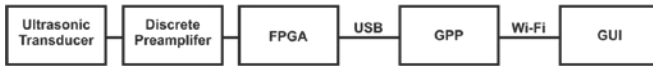
Fig. 4. Newly Developed Ultrasonic Acquisition Structure. All ultrasonic data, and co-incidentally all robot variables, are transferred wirelessly back to a computer base station GUI.
