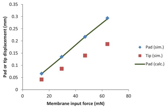
**Fig. 10.** Simulated pad and tip displacements for pressure loading of the pad at values shown in Fig. 4. Solid line shows calculated pad displacement (using Equation (1)) for each of the simulated tip displacements.
