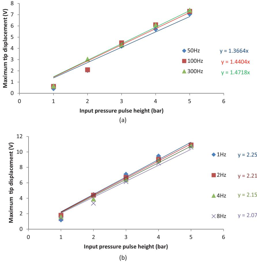
**Fig. 11.** (a) Effect of frequency on unloaded cantilever system compliance at higher frequencies (data from Fig. 4), (b) effect of frequency on unloaded cantilever system compliance at lower frequencies (data from Fig. 4).
