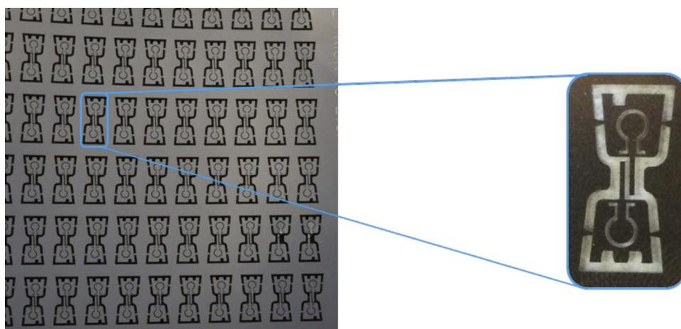
**Fig. 3.** Array of photo etched micro-grippers (scale bar 15 mm).
