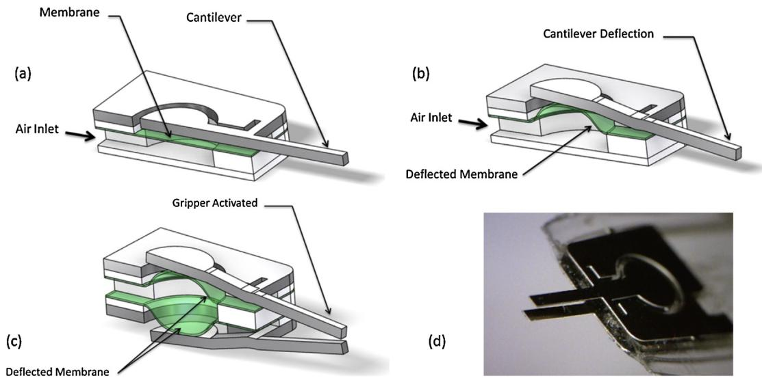
**Fig. 1.** Schematic drawings of working principle of the gripper device (a–c), and picture of assembled micro-gripper (d).
