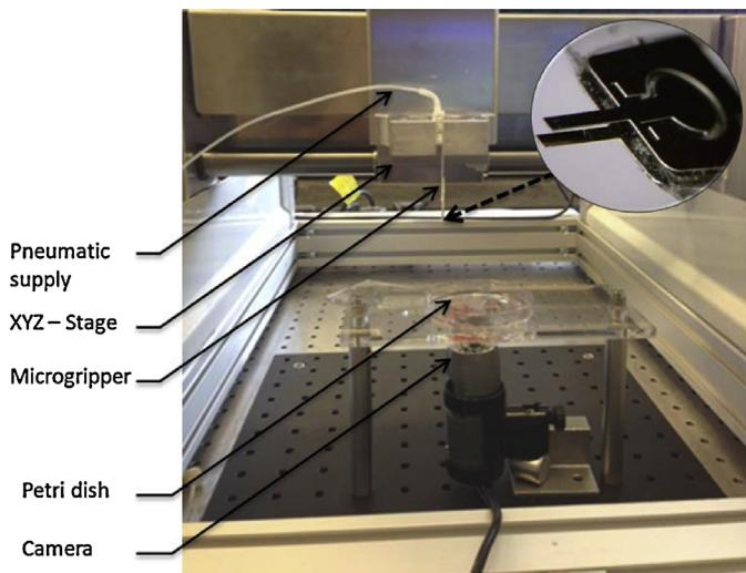
**Fig. 15.** Experimental setup for pick-and-place demonstration.
