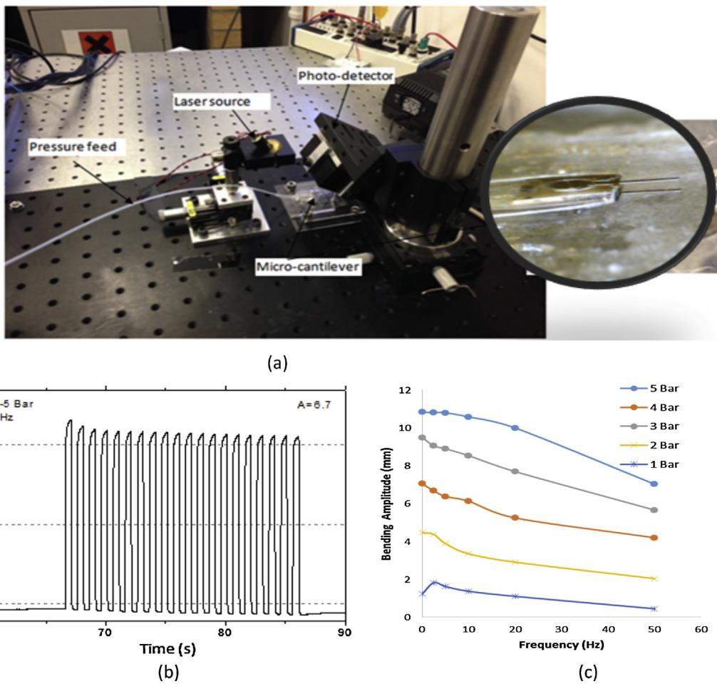
**Fig. 4.** (a) Dynamic test set-up with optical sensor, (b) Typical dynamic test output from optical sensor, (c) amplitude of tip displacement as frequency is varied for different pulsed pressures.
