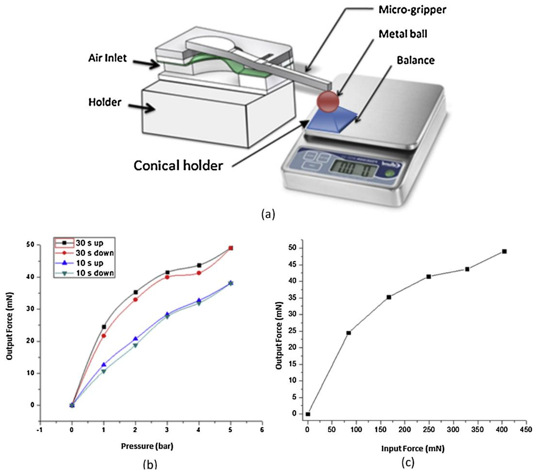
**Fig. 6.** (a) Schematic test set-up for static loading of cantilever), (b) Measured cantilever tip (output) force vs. input pressure, (c) Measured input and output forces at pressures used in (b) with 30 s dwell time.
