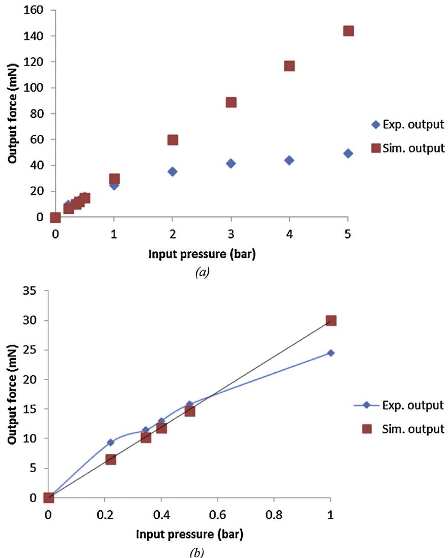
**Fig. 14.** Measured and simulated aoutput forces for a range of input pressures (a) range from 0 to 5 bar, (b) range from 0 to 1 bar.
