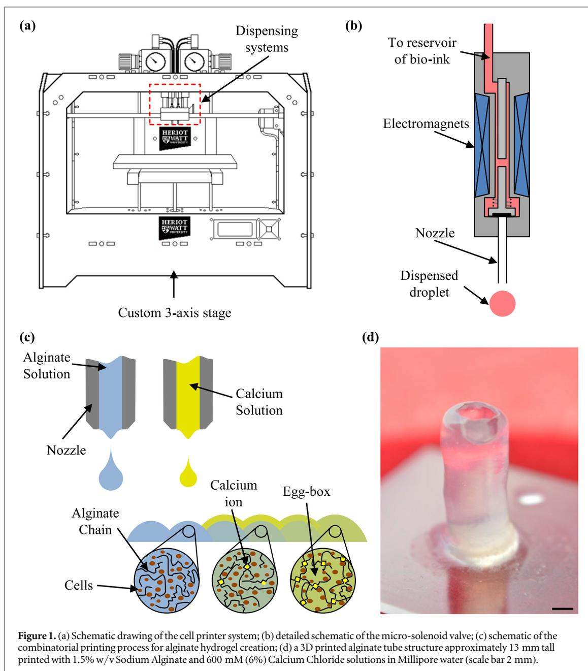
**Figure 1.** (a) Schematic drawing of the cell printer system; (b) detailed schematic of the micro-solenoid valve; (c) schematic of the combinatorial printing process for alginate hydrogel creation; (d) a 3D printed alginate tube structure approximately 13 mm tall printed with 1.5% w/v Sodium Alginate and 600 mM (6%) Calcium Chloride solutions in Millipore water (scale bar 2 mm).
