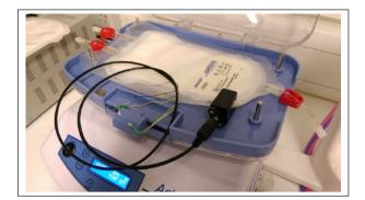
**Figure 6.** Final configuration of the sensor clip prototype integrating with HemoSep's<sup>®</sup> pre-existing technology. The current sensor can be connected to a standard 5V power supply via the red and black leads and the red and green LEDs for user visual feedback are connected to the clip via a cable.
