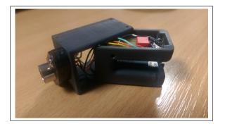
**Figure 1.** 3D-printed clip built in two parts to house the electronic components.
