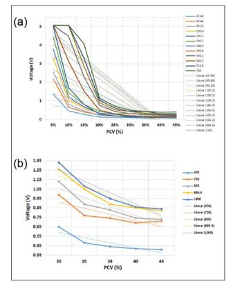
**Figure 3.** Voltage response of the sensor using various external resistors: a) 12 external resistors between 47.84k $\Omega$  and 720k $\Omega$  at the 5-45% PCV range and b) 5 higher value external resistors (between 470 k $\Omega$  and 1000 k $\Omega$ ) at the 30-43% range. Linear trend-lines were added to ascertain the steepest gradient. The highest resistor values tested displayed the greatest voltage delineation at these PCV values.
