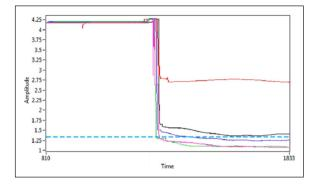
**Figure 5.** Voltage response acquired when placing varying blood concentration samples in the sensing circuit. The 4.23V baseline amplitude decreased to a greater extent as the blood concentration of the samples increased. The comparator reference voltage was set at 1.35V which corresponded to a PCV greater than 35%.
