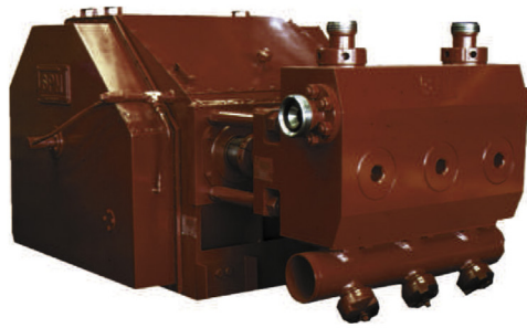
Fig. 7. Left image shows typical 3-cylinder positive displacement pump employed in hydraulic fracturing [53]. To the right, the table details the performance specification of a typical pump.
